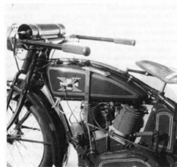
View showing striping on tank, forks, tool box, chain guard and frame.
