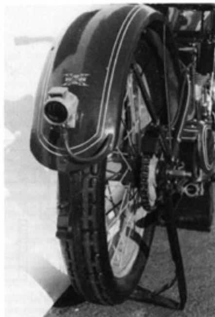
Gas tail lamp, small gold "X" decal and striping on rear guard.
