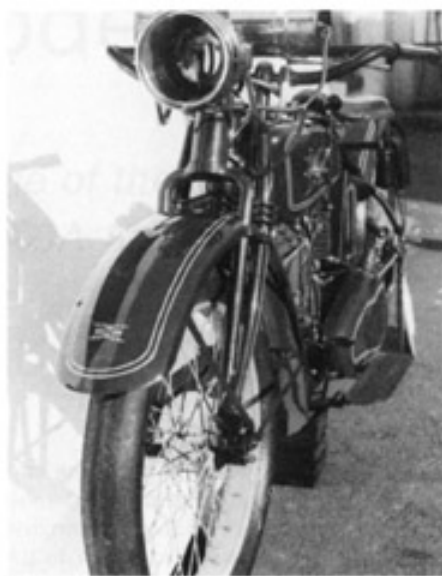
Front view showing wide mudguards, with double gold striping and small "X" Excelsior transfer supplied by restorer Hodgdon from his collection.
